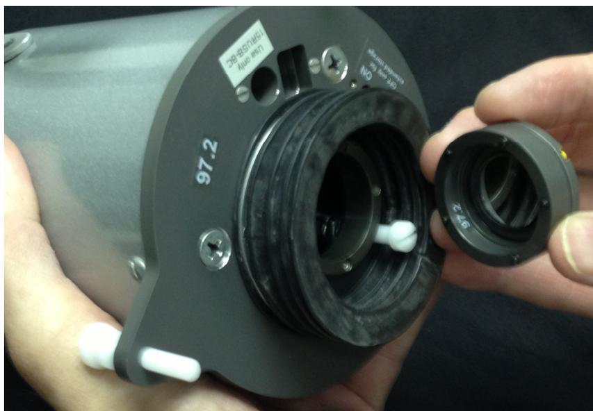
4. Calibrate the instrument. Adjust the reading with the gain knob to match the reflectance value for the standard. The reflectance value is found on the standard and on the base of the instrument. After
