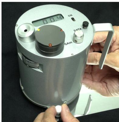
7. Maximize the reading by adjusting the outer legs. The maximum reading is the reflectance reading.
