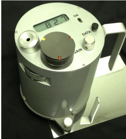
8. Moving the instrument to another spot on the test mirror the outer legs should already be close and require very little adjustment.
