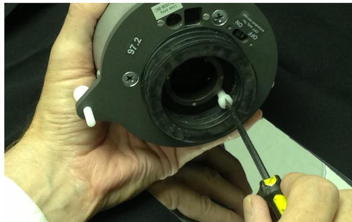
6. Place the 15R on the test sample. Adjust the outer legs to locate the reflected image within the aperture by watching for a reading on the display.
