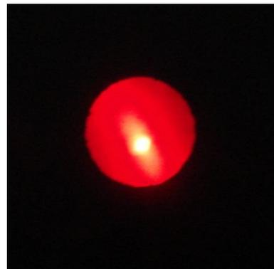
The tissue scatters light to provide illumination of the aperture edge and reduces the intensity of the source image. Note that the image of the source pinhole need not be perfectly centered in each aperture. Due to mechanical limitations the image will possibly be off center in each aperture and not off in the same direction.
