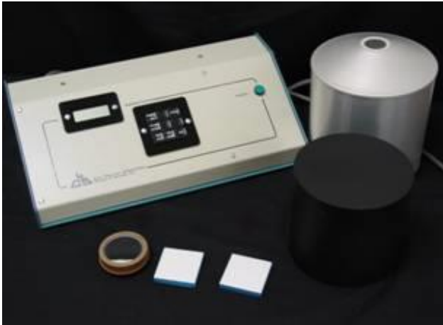
The SSR-ER version 6 Electronics Package and Measurement Head and calibration standards
