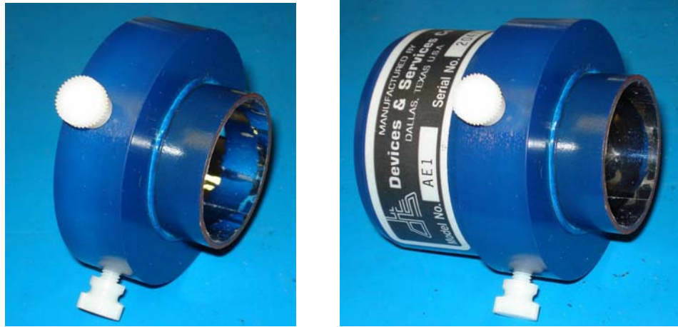
Standard AE-ADP adapter with highly reflective film that redirects radiation heat exchange
