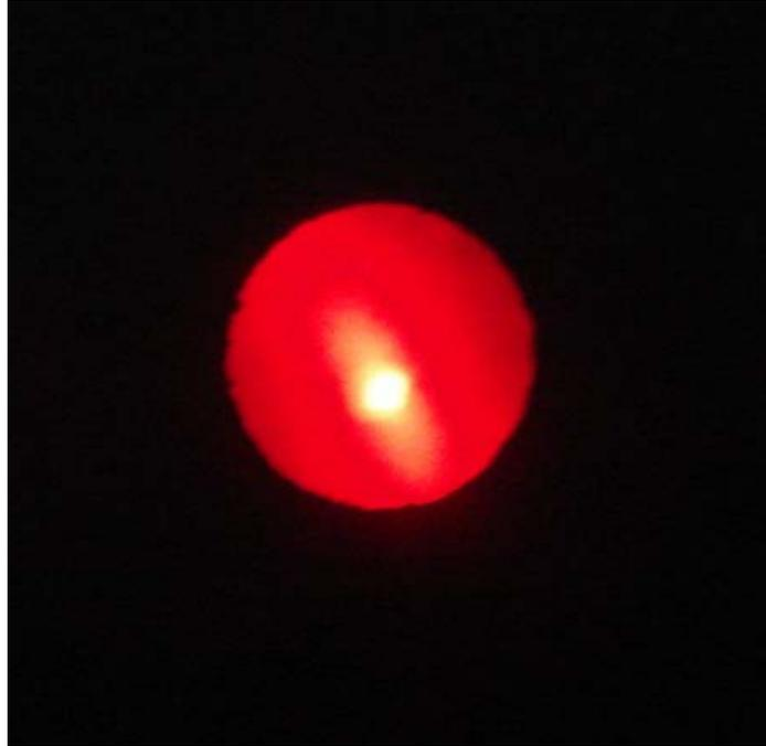
Note that the image of the source pinhole need not be perfectly centered in each aperture. Due to mechanical limitations the image will possibly be off center in each aperture and not off in the same direction.
