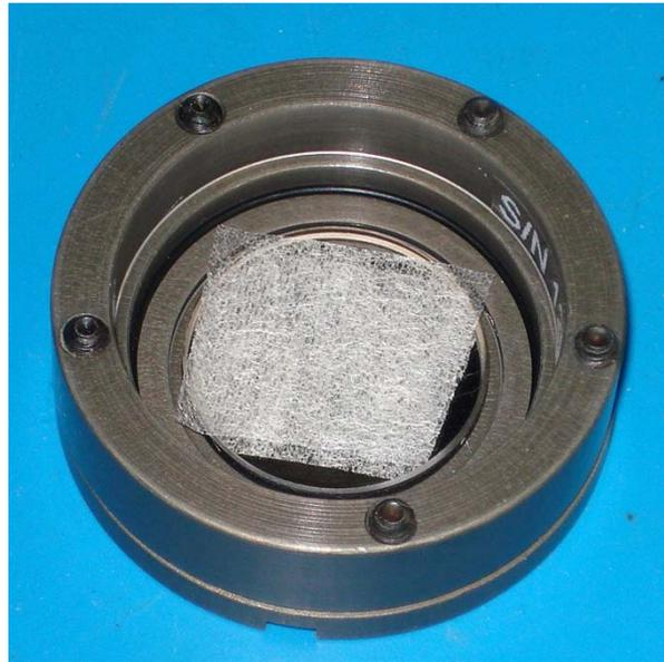
The tissue scatters light to provide illumination of the aperture edge and reduces the intensity of the source image. The reflected image with the tissue in place appears as shown below.
