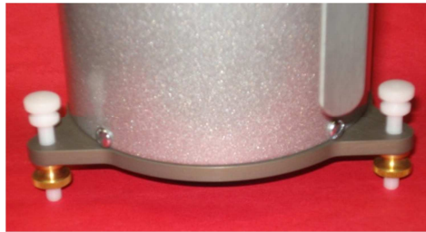
Photo showing locking hardware installed
