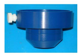
Emittance measurements with the Emissometer Model AE1 and the AE-AD3 adapter can be made on flat areas as small as approximately 0.9 inches (2.3 cm.) in diameter. Typical applications include making measurements on a small sample coupon of a material, and measuring a small available flat area on a larger sample. The adapter will clear a vertical obstruction up to 1 inch in height around the area to be measured.
